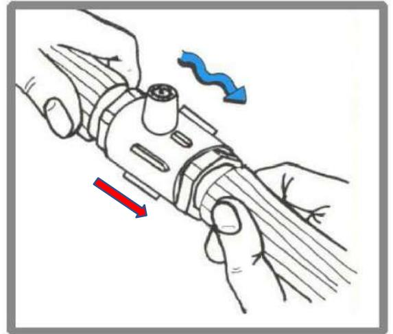
If it is necessary to insert the anti-syphon unit in any point of the outlet hose, use this type of valve, equipped with two universal hose connectors placed at the valve body ends.
