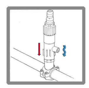
A polypropylene air intake which prevents any risk that the washing machine or dishwasher continuously drains due to the vacuum effect caused by the drainage pipe.
