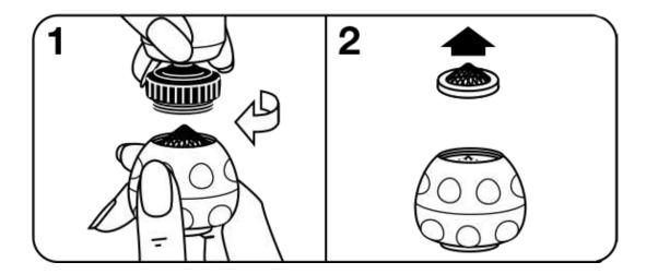
To keep the tap sprayer always in perfect conditions (even in case of irregular flow), clean the special stainless steel screenwasher.
