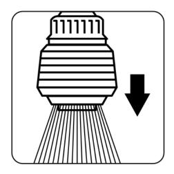
To switch the function of the tap sprayer (from aerator to shower), simply push the outer collar downwards.
